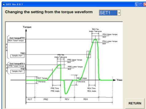
Fig. 4-7. Changing the setting from the torque waveform
