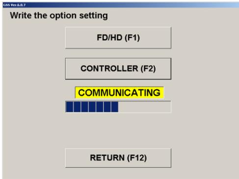
Fig. 4-14-43. Progress of writing to the controller
