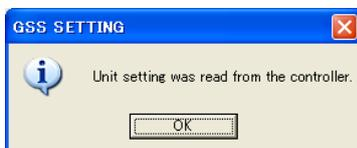
Fig. 4-14-25. Message for successful completion of loading the data from the controller
