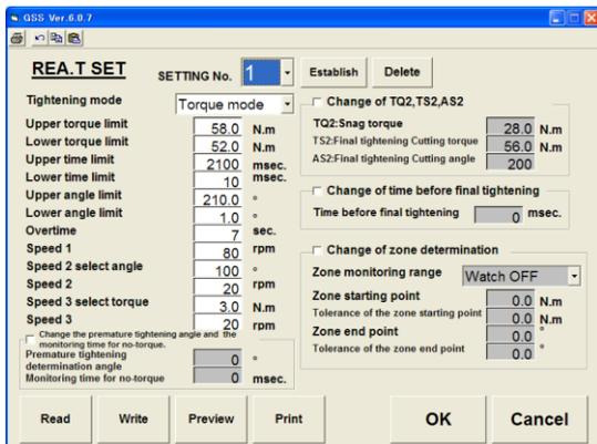
Fig. 4-6-2. Final tightening setting Torque method
