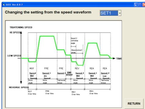
Fig. 4-8. Changing the setting from the speed waveform
