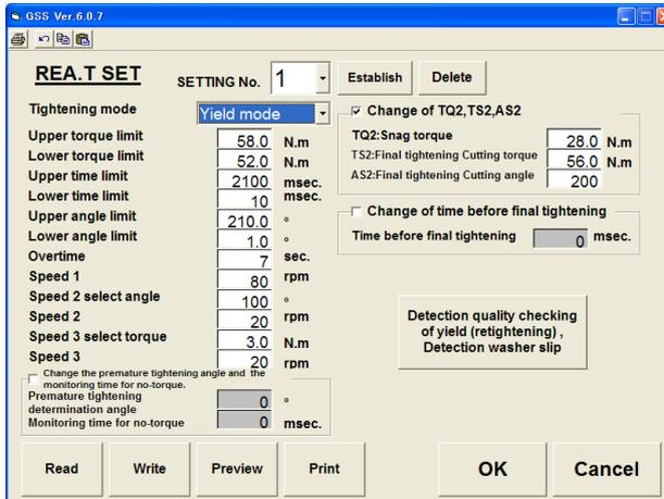
Fig. 4-6-4. Final tightening setting Yield method -(1)
