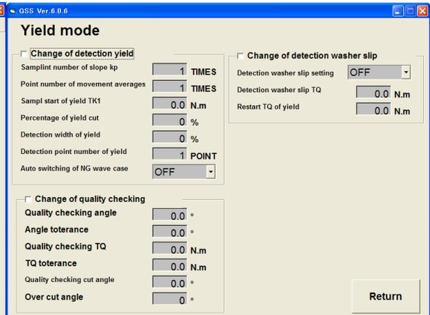
Fig. 4-6-5. Final tightening setting Yield method -(2)
