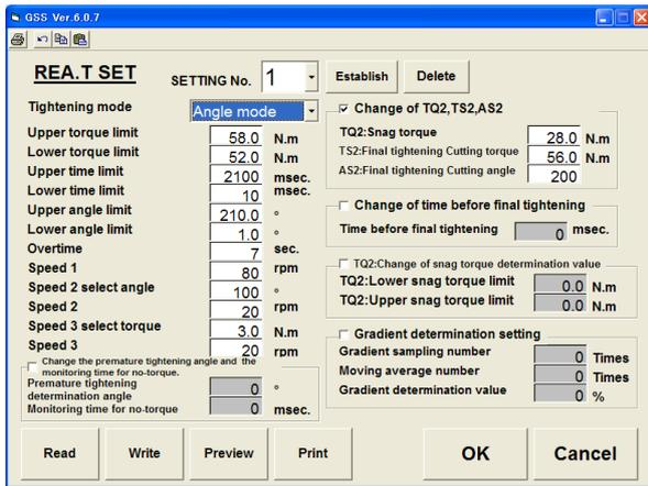
Fig. 4-6-3. Final tightening setting Angle method
