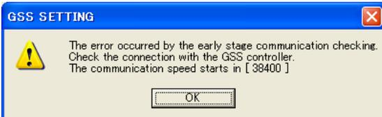
Fig. 1-3. Initial communication check error
